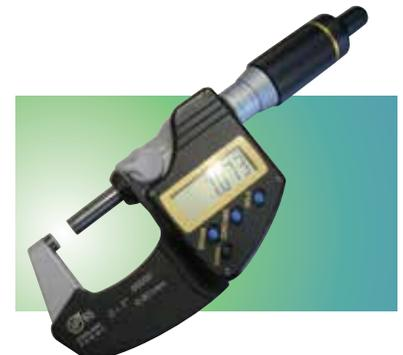
Figure 2b. Standard Micrometer
