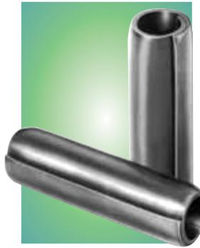
The use of a **Series 550 Cosmetic Coiled Pin** will simplify design as misalignment of the inner and outer holes to provide friction is no longer necessary. Intentional misalignment is difficult to control in production and induces stress in the hinge area causing cracking and pin fallout. Below are some guidelines that should be followed when designing cosmetic cases:
