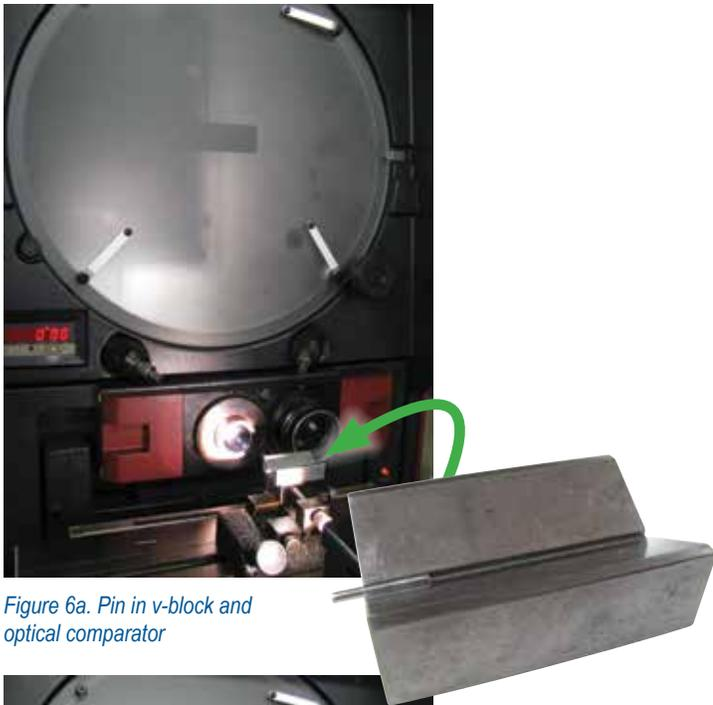
Figure 6a. Pin in v-block and optical comparator
