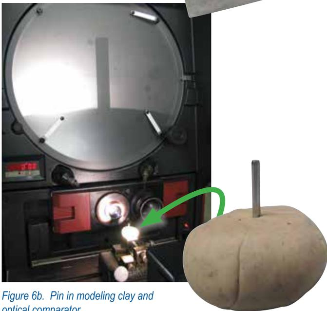
Figure 6b. Pin in modeling clay and optical comparator
