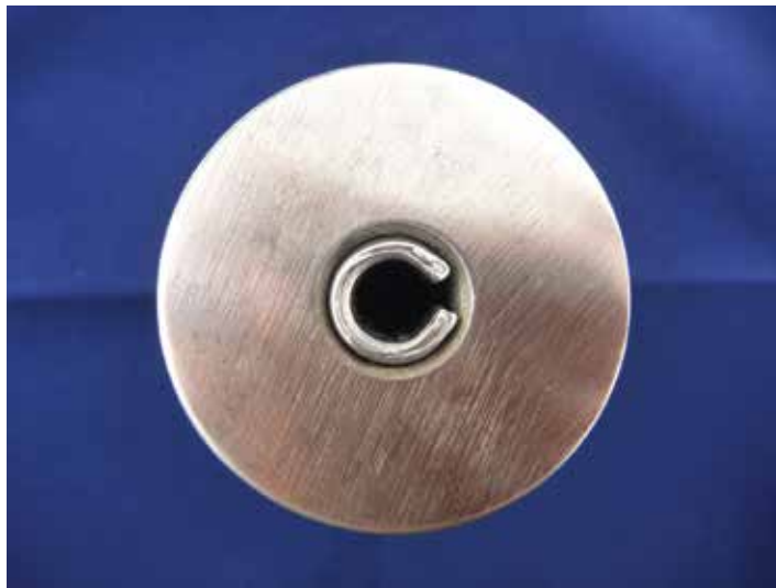
Figure 6: Slotted Pin installed in a oversized hole.
