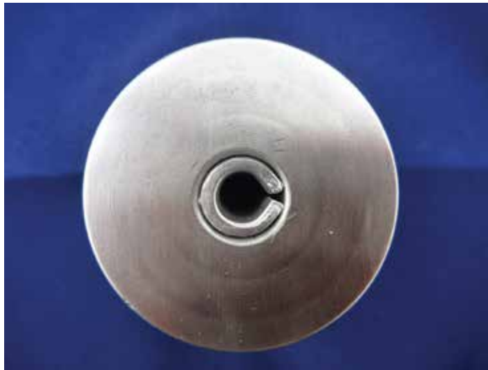
Figure 5: Slotted Pin installed in a nominal recommended hole. Notice the gap is virtually closed along the inside diameter of the pin.
