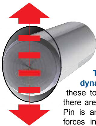
The Solid Pin's rigidity elongates the hole.
