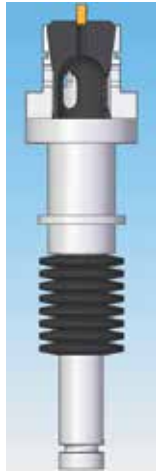
Left: Disc Springs are compressed, collet is open. Right: Disc Springs are uncompressed, collet is closed, work piece is clinched.
