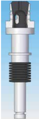
Left: Disc Springs are compressed, collet is open. Right: Disc Springs are uncompressed, collet is closed, work piece is clinched.
