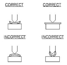
Micro-hardness testing of a coiled pin is the preferred method. To test using this method, the pin is cross-sectioned and one of the resultant pieces mounted for test. The mount is then polished to remove cutting marks. It is critical to note that the cutting and polishing operations must be performed with proper coolants to prevent excessive heating of the sample.
