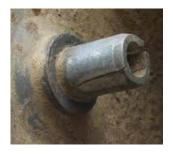
hole. This causes stress to concentrate 180° from the slot. Over time, this weak area was exacerbated by impact loads, leading to failure. The Slotted Pin was at risk to fall out of the hole and the productivity and safety of the construction site was compromised.
