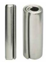
There are two distinct types of Spring Pins: Coiled Spring Pins and Slotted Spring Pins. Both types share certain characteristics such as flexibility and their ability to accommodate wider hole tolerances than nonflexible fasteners (such as Solid Pins). However there are a few major differences between the two types of Spring Pins that must be understood - particularly for medical device manufacturers.
