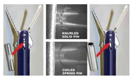
The knurled Solid Pin generated debris during insertion into surgical "grasper". The Coiled Spring Pin installed cleanly.
