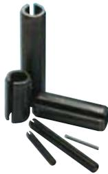
As a Slotted Pin is installed, the pin’s “spring like” characteristic is reduced to a narrow stress seam opposite to the slot. Here, **stress concentrations** form as a result of the pin’s limited flexibility. This portion of the Slotted Pin is susceptible to failure if the pin is subject to impact loads.
