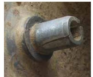
hole. This causes stress to concentrate 180° from the slot. Over time, this weak area was exacerbated by impact loads, leading to failure. The Slotted Pin was at risk to fall out of the hole and the productivity and safety of the construction site was compromised.
