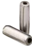
A second mode of failure is caused by the Slotted Pin’s rigidity after installation. When a Slotted Pin is installed, the slot closes and the pin can act like a rigid hollow tube. This tube behaves similarly to a Solid Pin. As a solid member, impact loads are transmitted to the host wall, causing **hole elongation**. As the hole size increases, impact loads intensify, and failure is accelerated. The pin cracks, falls out of the hole, or does both.
