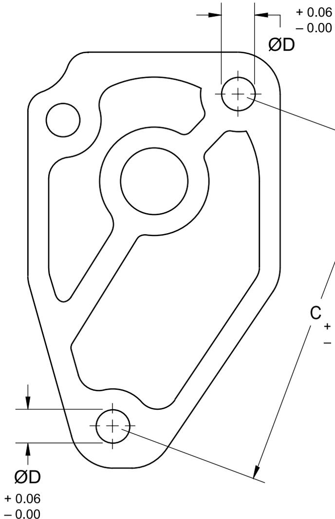
If more than one Dowel is used, centreline tolerancing for hole positioning becomes an issue. In situations with precision holes requiring precision locating, the centreline tolerancing needs to be accurate and similar to tolerancing used for solid Dowels. A tolerance of .0006" or 0.015 mm is recommended. When a Dowel is installed in a minimum hole, which is recommended in these cases, the Dowel gap is butted and further spring action is very limited, if any.
