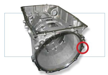
An OEM was using a 16mm OD Ground Solid Dowel to locate the transmission to the back of the engine. This particular application was more demanding than most due to the weight of the two components to be aligned and the method of joining them together. The customer approached **SPIROL** for cost-reduction suggestions.
