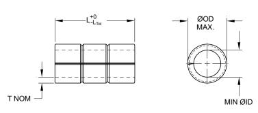
Parts less than 20mm (.750") long will have a single groove.
