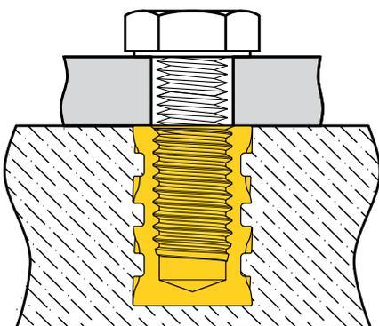
Blind-end Inserts provide an additional alternative to prevent plastic from flowing into the inside of the Insert.
