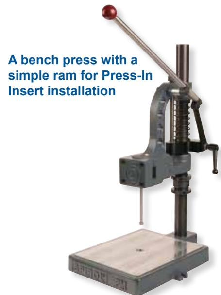
A bench press with a simple ram for Press-In Insert installation
