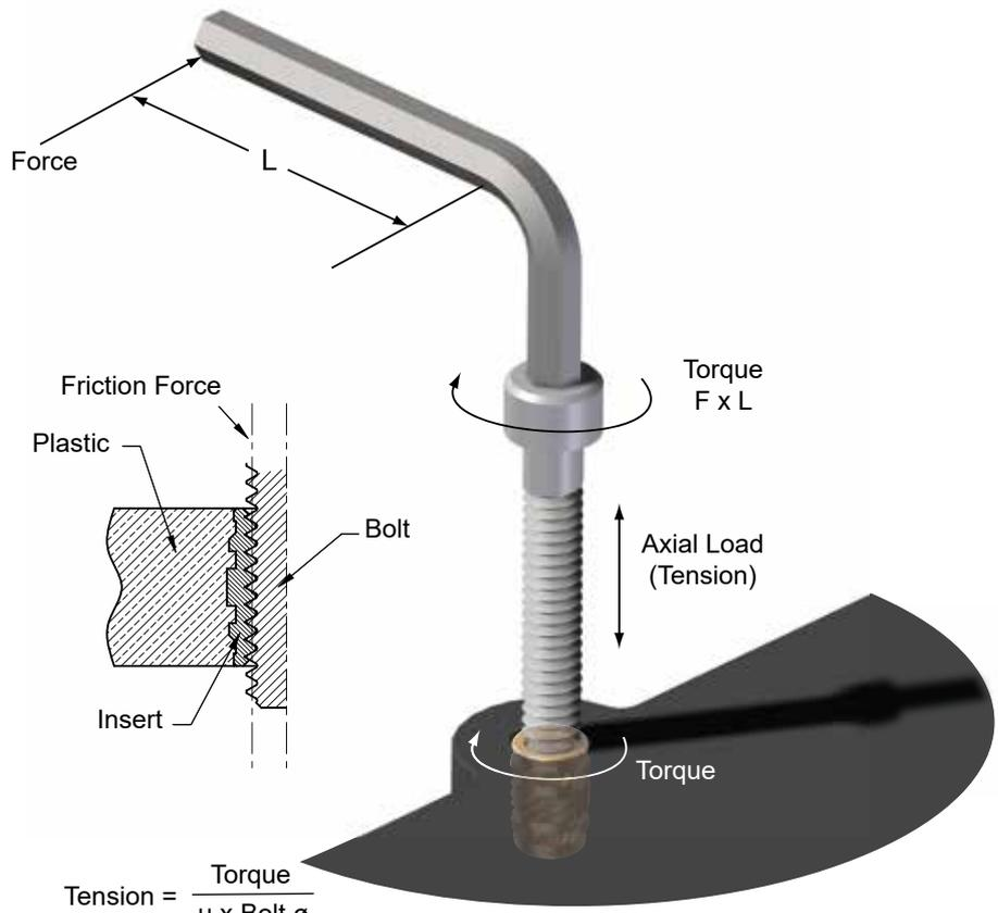
$$\text{Tension} = \frac{\text{Torque}}{\mu \times \text{Bolt } \phi}$$
