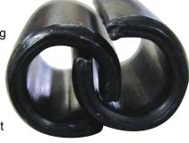
Example of interlocked Slotted Pins
