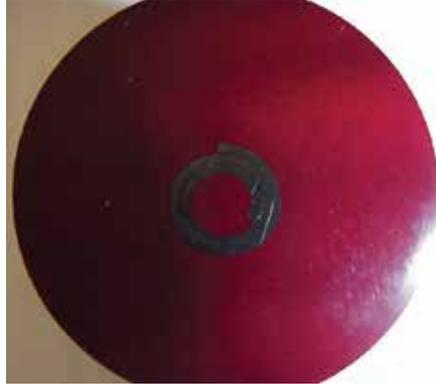
*Photograph of a mounted and polished coiled spring pin.
