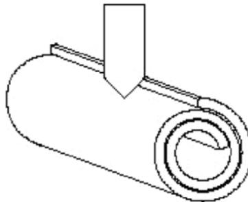
REMOVE TEST STRIP PERPENDICULAR
