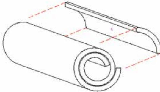
\*Note 'X' marks correct test location at center of strip.
