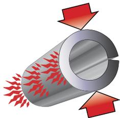
As a result of the pin’s limited flexibility. This portion of the Slotted Pin is susceptible to failure if the pin is subject to impact loads.
