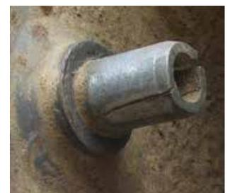
hole. This causes stress to concentrate 180° from the slot. Over time, this weak area was exacerbated by impact loads, leading to failure. The Slotted Pin was at risk to fall out of the hole and the productivity and safety of the construction site was compromised.
