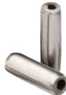
A second mode of failure is caused by the Slotted Pin’s rigidity after installation. When a Slotted Pin is installed, the slot closes and the pin can act like a rigid hollow tube. This tube behaves similarly to a Solid Pin. As a solid member, impact loads are transmitted to the host wall, causing **hole elongation**. As the hole size increases, impact loads intensify, and failure is accelerated. The pin cracks, falls out of the hole, or does both.
