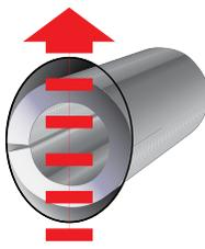
Direction of impact load and resulting hole elongation.
