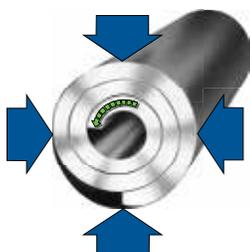
The solution to these problems is **SPIROL’s Coiled Pin**. As the Coiled Pin is installed, stress is distributed throughout the fastener instead of being concentrated along a line. The Coiled Pin’s design also ensures **flexibility after installation**. For the life of the assembly, the Coiled Pin is able to absorb impact
